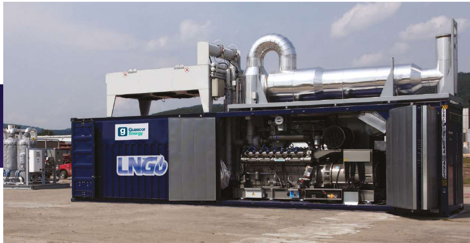
LNGo micro-scale natural gas liquefaction system.
